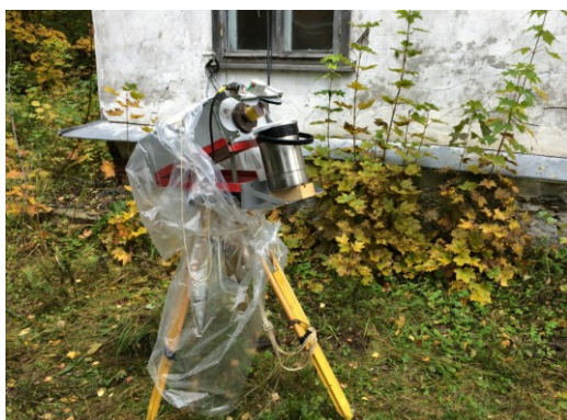
Figure 1. General view of a mobile microwave ozonemeter. Parameters of device: observation frequency – 110.8 GHz ; temporal resolution – 15 min ; band of the analysis of a spectrometer – 240 MHz ; frequency resolution – from 1 up to 10 MHz ; in measurements of spectra of a middle atmosphere ozone the method of absolute calibration is used; estimation of a vertical profile of ozone at altitudes from 20 up to 60 km is carried out accuracy of 10–15% .
