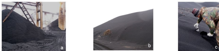
Figure 9. Pechenganickel fresh granular slags (a), mature slag dump (b), sampling of undisturbed slags (c)
